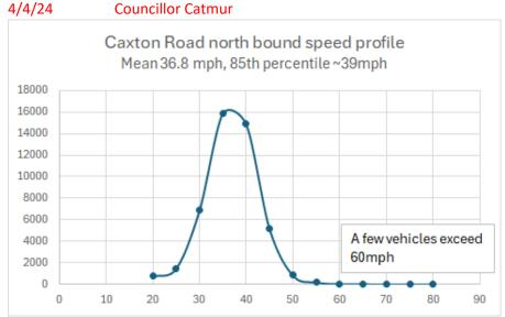
A graph of the data collected on CAXTON Road near the nursery footpath crossing, sample size 46,128 vehicles, using the MVAS in 'no display mode' and removing vehicles entering the industrial site (they tend to be less than 20mph)
